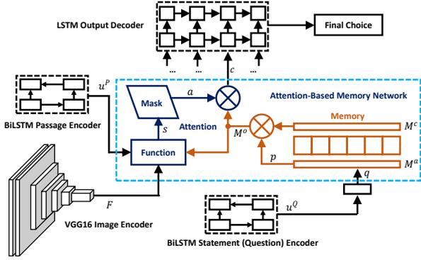
Figure 4: The attention-based memory network in our model. The encoded statement is made as a query to visit the memory to obtain the memory output. The attention mechanism combines the encoded passage and image to generate a mask acting on the memory output. The latent features of all the options for a question are aggregated orderly to find the final choice by an LSTM decoder.
