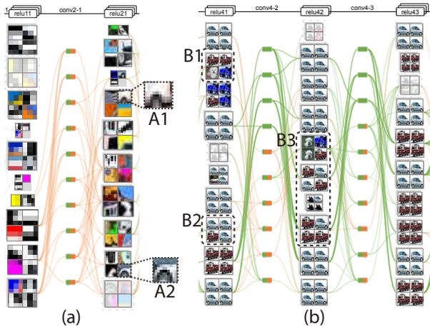
Fig. 10. Learned features of BaseCNN: (a) low-level feature; (b) high-level features.
