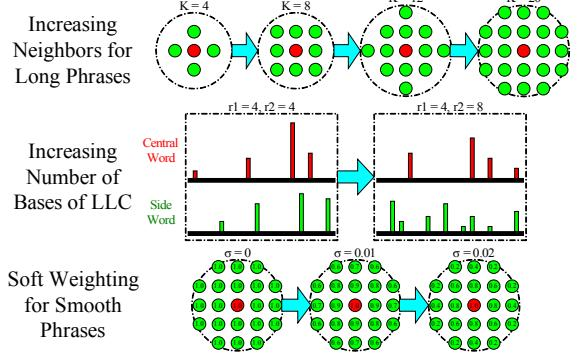
Figure 9: Illustration of different improvements for GPP (best viewed in color PDF). Above: increasing  $K$  for long phrases. Middle: Enlarging number of bases in LLC for more overlapping. Below: Soft weighting on geometric visual phrases, where floating numbers are the soft weights on visual words.
