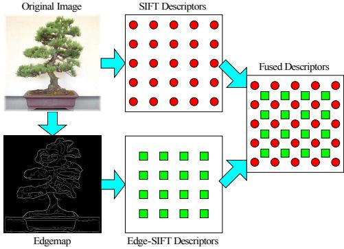
**Figure 2:** Fusing two categories of dense descriptors on the image plane.
