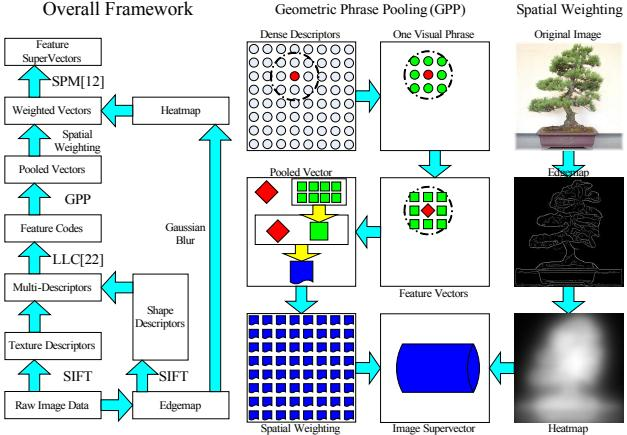
**Figure 1:** Flowcharts and of the framework and key modules. Left: the modified BoF framework. Right: Geometric Phrase Pooling and spatial weighting.
