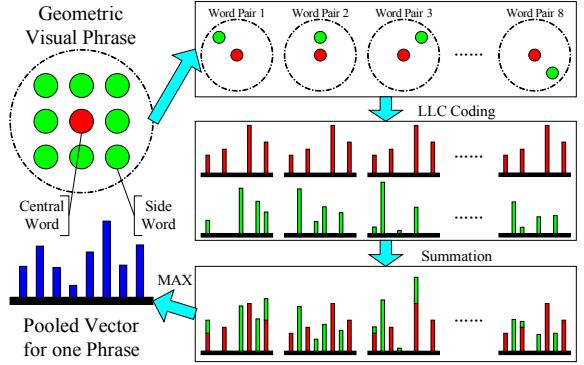
Figure 6: Illustration of Geometric Phrase Pooling. We group the central word and each side word as a pair and add their feature vectors together. At last, maximization is performed on the whole phrase.
